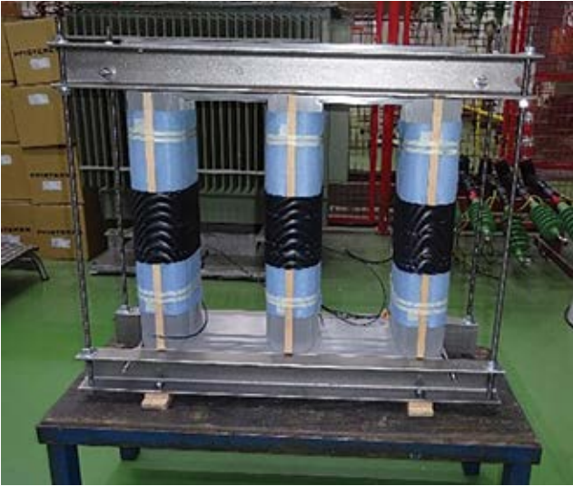
Laboratory scale experimental setups by SGB-SMIT Group to validate core losses improvement
